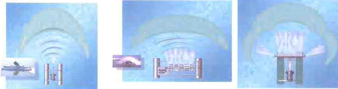
Figure 4 – Various pontoon mounted aeration devices showing the sludge mounds generated by the high horsepower water thrust. These sludge mounds deflect water mixing movement across the rest of the lagoon bottom.
